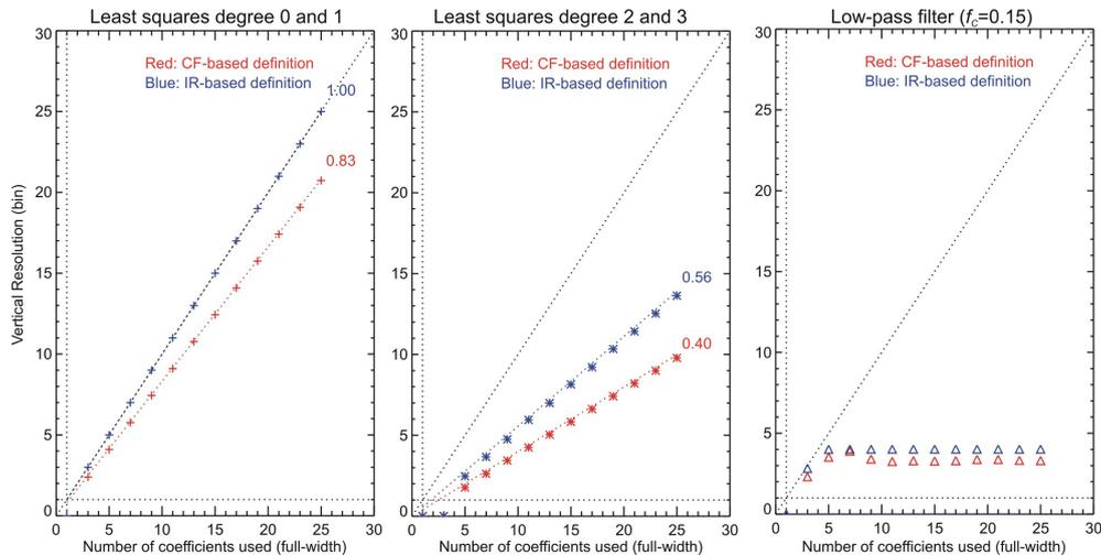
**Figure 13.** Correspondence between cut-off frequency-based (red) and impulse-response-based (blue) vertical resolution (in bins), and the number of filter coefficients used (full width), for three filters introduced in Sect. 2. The dashed gray line represents unity slope (i.e., one bin for one point), and the numbers at the end of the red and blue dotted straight lines indicate the slope of the linear fit applied to the paired points for each definition.
