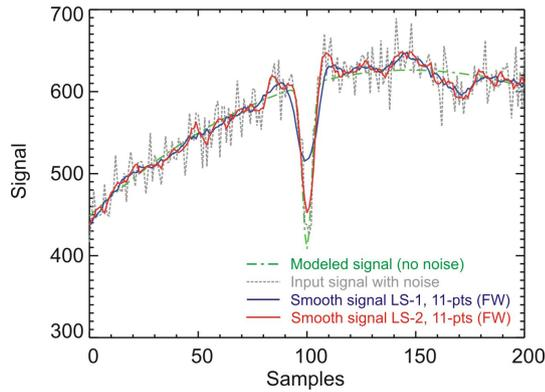
**Figure 1.** Example of the differing impact of two smoothing filters of identical number of terms ( $2N + 1 = 11$ ). The green dash-dotted curve is the modeled signal (with no noise), the gray dotted curve is the modeled input signal containing Poisson noise, the blue and red curves are the smoothed signal using an 11-point boxcar average (LS-1), and the least-squares fitting method with a polynomial of degree 2 (LS-2), respectively.
