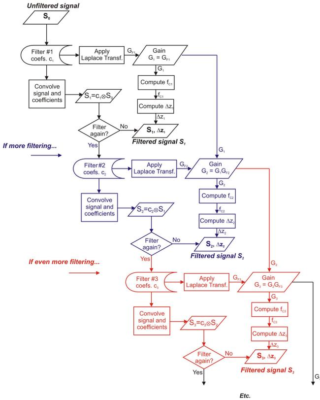
**Figure 9.** Schematics summarizing the procedure that should be followed to compute the standardized vertical resolution with a definition based on cut-off frequency when the signal or profile is filtered multiple times.
