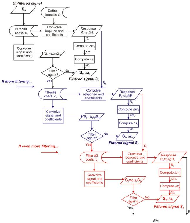
**Figure 7.** Schematics summarizing the procedure that should be followed to compute the standardized vertical resolution with a definition based on impulse response when the signal or profile is filtered multiple times.
