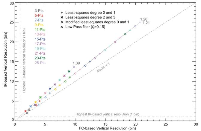
**Figure 10.** Comparison between the cut-off frequency-based and the impulse-response-based standardized vertical resolutions for several smoothing filters introduced in Sect. 2 and in the Supplement. The numbers at the end of the dotted straight lines indicate the proportionality constant (slope) between the two definitions for three of the four types of filters used. There is no such proportionality for the low-pass filter (prescribed cut-off frequency).
