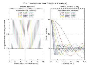
**Figure 2.** Impulse response (left) and gain (right) for a digital filter equivalent to fitting an unsmoothed signal with a polynomial of degree 1 or 2 using the least-squares method over an interval comprising 2N + 1 points (full width). Full widths represented in this figure range from 3 to 25 points. This least-squares filtering procedure is equivalent to a running average over 2N + 1 points (full width).
