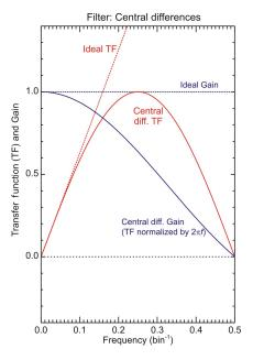
**Figure 4.** Transfer function (TF) and gain of the central difference digital filter. The gain (blue curve) is the transfer function (red curve) normalized by  $2\pi f$ , which is the real part of the ideal differentiator  $i\omega$ .
