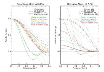
**Figure 5.** Transfer function (gain) of several smoothing (left) and derivative (right) filters, all with exactly the same number of coefficients, 2N + 1 (five-point full width for the smoothing filters and seven-point full width for the derivative filters).
