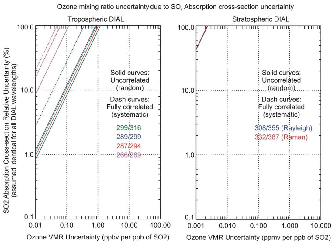
5 **Figure 10: Ozone mixing ratio uncertainty as a function of SO<sub>2</sub> cross-section relative uncertainty (%) assuming that all cross-sections used have the same relative uncertainty. Solid curves are used for cases of independent (“random”) cross-section datasets, and dashed curves are used for the case of full correlation between all cross-sections.**
