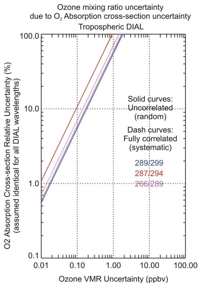
5 Figure 11: Ozone mixing ratio uncertainty as a function of O<sub>2</sub> cross-section relative uncertainty (%) assuming that all cross-sections used have the same relative uncertainty. Solid curves are used for cases of independent (“random”) cross-section datasets, and dashed curves are used for the case of full correlation between all cross-sections.
