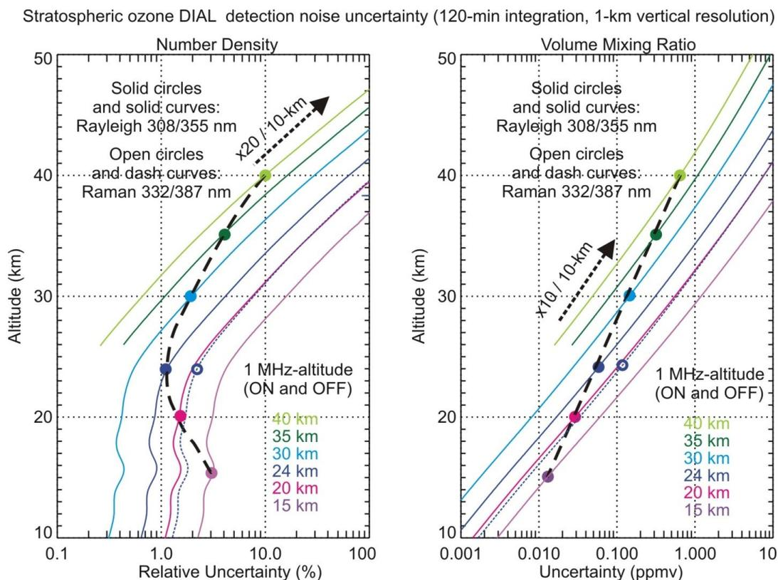
5 **Figure 1: Ozone number density relative uncertainty (left) and ozone mixing ratio uncertainty (right) owed to detection noise for stratospheric ozone DIAL systems of varying performance, and for a 120-minutes integration time and 1-km vertical resolution. The systems' performance is measured as the altitude of 1-MHz count rate for both the ON and OFF channels signals. See text for details.**
