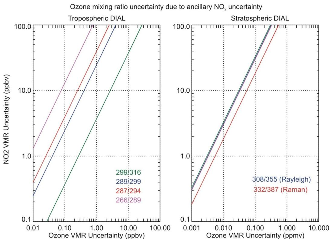
Figure 12: Ozone mixing ratio uncertainty as a function of NO<sub>2</sub> mixing ratio uncertainty (ppbv). Left plot: Tropospheric ozone DIAL pairs (uncertainty in ppbv); Right plot: Stratospheric ozone DIAL pairs (uncertainty in ppmv).
