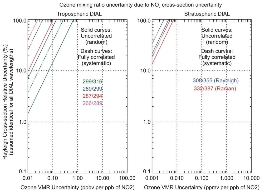
5 **Figure 9:** Ozone mixing ratio uncertainty as a function of NO<sub>2</sub> cross-section relative uncertainty (%) assuming that all cross-sections used have the same relative uncertainty. Solid curves are used for cases of independent (“random”) cross-section datasets, and dashed curves are used for the case of full correlation between all cross-sections).
