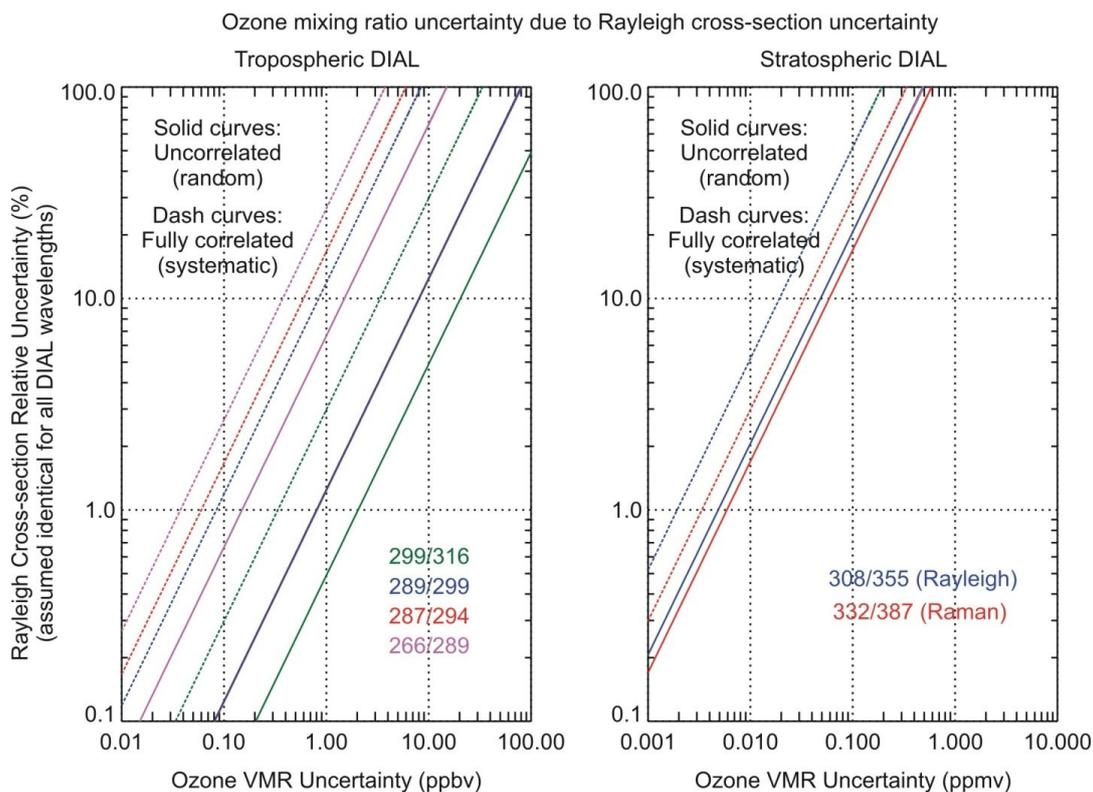
5 **Figure 8: Ozone mixing ratio uncertainty as a function of Rayleigh cross-section relative uncertainty (%) assuming that all cross-sections used have the same relative uncertainty. Solid curves are used for cases of independent (“random”) cross-section datasets, and dashed curves are used for the case of full correlation between all cross-sections.**
