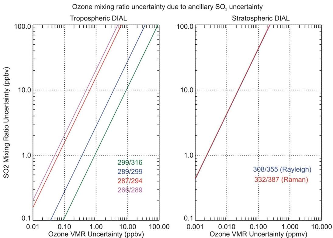
Figure 13: Same as Fig. 12, but for interfering gas SO<sub>2</sub>.
