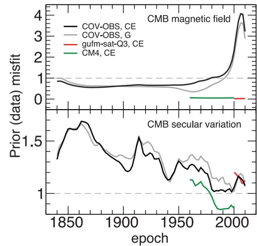
**Figure 2.** Normalized misfits to the data (prior misfits)  $\Delta_B$  (top) and  $\Delta_{\dot{B}}$  (bottom, see text for definitions), obtained by inverting models COV-OBS, gufm-sat-Q3 and CM4 with priors CE and G. A misfit of 1 (dashed grey line) denotes an acceptable fit (0 is optimal).
