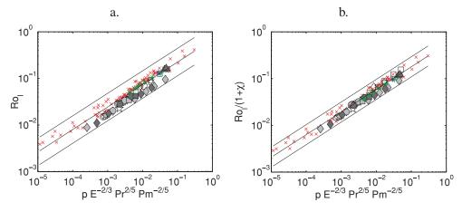
**Figure 8.** Local Rossby number  $Ro_l$  as a function of the combination  $pE^{-2/3}Pr^{2/5}Pm^{-2/5}$  proposed in Olson & Christensen (2006). (a) Without a dependence in  $\chi$ , (b) with a dependence in  $\chi$ . Symbols as in Fig. 3. Our data set is filtered to exclude the non-dynamo run.
