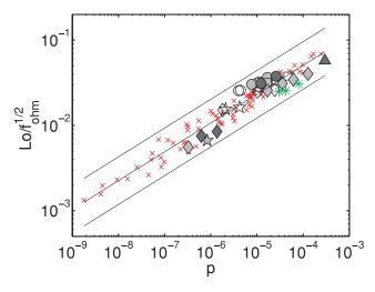
**Figure 4.** Dimensionless magnetic field, or Lorentz number *Lo*, corrected with the ohmic dissipation fraction  $f_{\rm ohm}^{0.5}$ , as a function of the dimensionless convective power *p*. Symbols as in Fig. 3. Our data set is filtered to exclude dynamos with a dipole fraction  $f_{\rm dip} \le 0.35$ .
