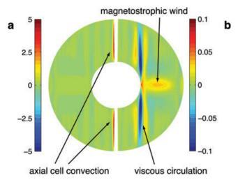
**Figure 4.** Meridional plane projection of the time and azimuthal average of (a) the radial velocity field  $u_r$ , and (b) the Coriolis torque integrand  $r^2 \sin^2 \theta \, u_r$  (eq. 8), for the case presented in Fig. 1(b). Amplitudes are normalized with  $u_{\varphi}$  in (a) and  $D^2 u_{\varphi}$  in (b).
