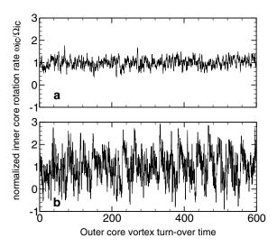
**Figure 6.** Time-series of the instantaneous inner core rotation rate  $\omega_{\rm ic}$ , normalized by its time-averaged value  $\Omega_{\rm ic}$ , for the runs presented in Fig. 1(a) (panel a) and 1(c) (panel b), which respectively have  $E=3\cdot 10^{-5}$  and  $E=3\cdot 10^{-6}$ . Time is normalized by the outer core overturn time D/U, where U is the root-mean-squared, time-averaged velocity in the fluid outer core
