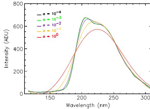
**Figure 2.** Effect of the Tikhonov regularization. Variation of the simulated NO spectrum as a function of the  $\alpha$  parameter. The greater the  $\alpha$  value, the smoother the convolved spectrum.
