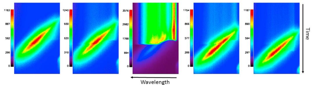
**Figure 1.** Example of representation of the five SPICAV bands. The color scale represents the intensity of the emission in Analogue-to-Digital Units (ADU). Each band is a tempo spectrum, with the wavelength on the x axis and the time on the y axis. The star signal is mainly visible on the central band. The red vertical line is the Lyman alpha stellar emission. An airglow—lenticular shape—is visible on every band.
