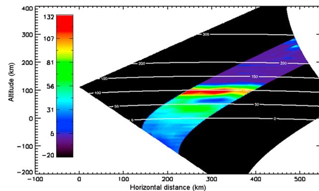
**Figure 4.** Image of the field of view created by the inversion algorithm for orbit 0267A10. A second emission zone is visible at tangent altitudes below the main airglow emission. The color bar expresses the airglow intensity in kR. The black color (value of  $-20$ ) indicates a lack of data.
