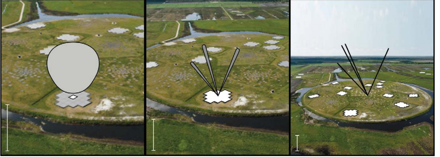
Fig. 1. Three successive zoom-outs showing the stations in the LOFAR core. The different scales of the hierarchically organised HBA elements are highlighted and their respective beam sizes are shown. The large circular area marks the edge of the Superterp, which contains the inner-most 6 stations (i.e. 12 HBA sub-stations: where there are 2 sub-stations, each of 24 tiles, in each HBA core station); other core stations can be seen highlighted beyond the Superterp in the third panel. Left: a single HBA tile and associated beam. Middle: a single HBA sub-station with three simultaneous station beams. Right: the 6 stations of the Superterp plus 3 core stations in the background are highlighted. Four independent beams formed from the coherent combination of all 24 core HBA stations, most of which are outside this photo, are shown. For the LBA stations, a similar scheme applies except that each LBA dipole can effectively see the whole sky. Fields of the relatively sparsely distributed LBA antennas are visible in between the highlighted HBA stations in all three panels.
