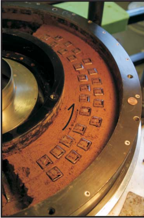
Figure 2. Plastic cubes pressed into the shear zone of the Douglas till after an experiment. The uppermost part of the till specimen has been removed to expose the shear zone. The width of the chamber of the ring shear device is 0.115 m. The solid black arrow indicates the direction of shearing (rotation direction of the rotating base).
