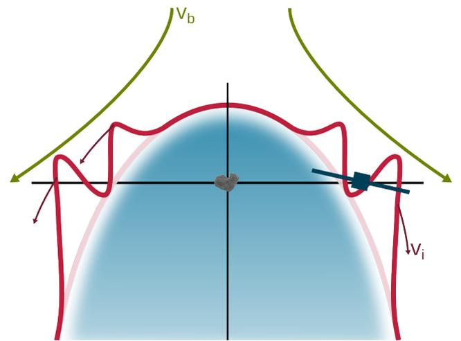
**Fig. 5.** Sketch of the magnetic field configuration in the frame where the ionopause (red) does not move. The lighter red line indicates the undisturbed cavity boundary. Rosetta's position is indicated in dark blue and the field free region is shaded in blue.  $v_i$  indicates the velocity of the instabilities and  $v_b$  the velocity of the ion bulk flow (green arrows).
