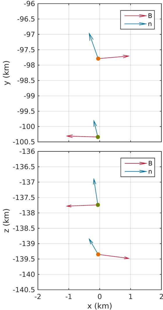
**Fig. 2.** Normal vector of the ionopause (blue) and averaged magnetic field (red) in the  $x - y$  plane (*top*) and the  $x - z$  plane (*bottom*) in CSEQ coordinates. The green point marks the inbound crossing, the orange point the outbound crossing. We note that the normal vector only indicates the direction and not the orientation of the boundary normal.
