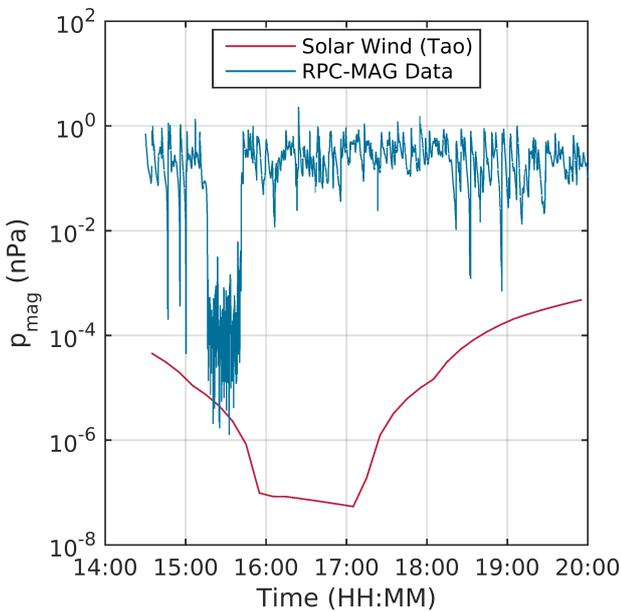
**Fig. 4.** Solar wind magnetic pressure obtained using the [Tao et al. \(2005\)](#) model and magnetic pressure as measured by RPC-MAG. The low-pressure region in the solar wind lasts from  $\sim 16:00$  to  $\sim 17:00$ . We note that to predict the solar wind magnetic field at the comet we used a simple one dimensional MHD model that has large uncertainties.
