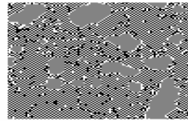
Figure 4b). Segregation (300 Mc cycles), A: white, B: black, V: grey (A=B = 40%, V= 20%, \varepsilon_{AA}=\varepsilon_{AB}=\varepsilon_{AV} =0.6 ; \varepsilon_{BB}=\varepsilon_{BV} =0.4 )
