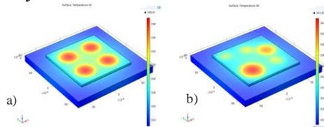
Figure 3: Temperature mapping with circular defects distributed in the ICM: a) regularly (radius 2.2 mm, porosity 40%), b) at random (maximum radius 1.8 mm, porosity 40%)
