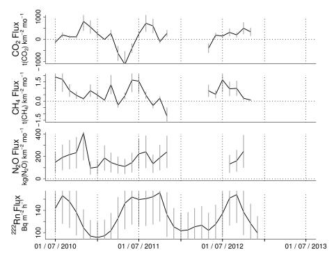
Figure 8. Monthly  $CO_2$ ,  $CH_4$  and  $N_2O$  fluxes at the Puy de Dôme station derived from the radon tracer method. The last panel presents the hourly  $^{222}$ Rn exhalation rate (U. Karstens and I. Levin, personal communication, 2014). The vertical grey lines are the respective flux uncertainties.
