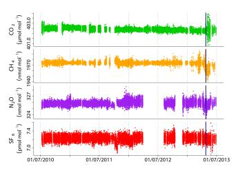
**Figure 4.** Time series of the target gas measured with the GC system at Puy de Dôme. The vertical blue lines in each panel correspond to the date of the working standards change.
