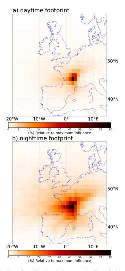
**Figure 1.** Footprint of the Puy de Dôme station from the Lagrangian dispersion model Flexpart (a) during daytime (14:00 to 16:00 UTC), when the PBL is usually well developed, and (b) during nighttime (22:00 to 06:00 UTC), when the station is usually in the free troposphere.
