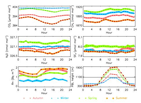
**Figure 6.** Mean diurnal cycles of CO<sub>2</sub>, CH<sub>4</sub>, N<sub>2</sub>O, SF<sub>6</sub>, and <sup>222</sup>Rn together with the planetary boundary layer height (relative to Clermont-Ferrand altitude – 396 m a.s.l.) at the Puy de Dôme station for each season. Trace gas mole fractions were detrended based on 1 January 2013.
