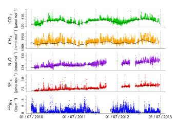
**Figure 5.** Hourly mole fractions of  $CO_2$ ,  $CH_4$ ,  $N_2O$  and  $SF_6$  atmospheric ambient air and hourly activities of  $^{222}Rn$  at Puy de Dôme from July 2010 to June 2013. The black lines are the respective monthly GHG background mole fractions of the Puy de Dôme measurements (between 22:00 and 06:00 UTC) and the  $^{222}Rn$  background activity at Mace Head (Ireland).
