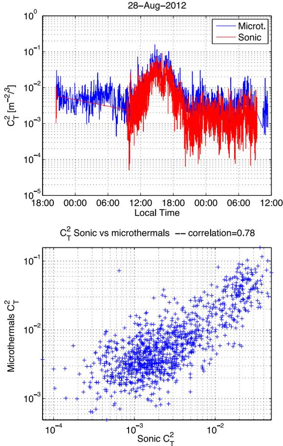
**Figure 7.** Simultaneous measurements of  $C_T^2$  at Nice observatory in 2012 August. Left: times series. Right: plot of sonic  $C_T^2$  versus microthermal  $C_T^2$  within coincidence intervals of 30 s.
