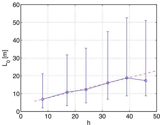
**Figure 6.** Outer scale  $L_0$  as a function of the height of the anemometer. Error bars are the intervals containing 50 per cent of the data. The dashed line is a least-squares fit obtained on the five first points.
