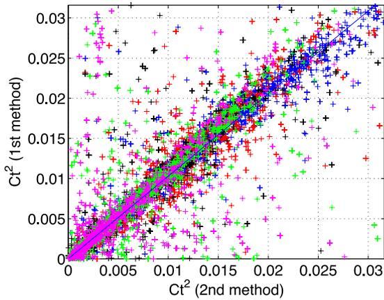
**Figure 5.** Comparison of  $C_T^2$  values computed from the first method (fit of the inertial domain of the structure function) and the second method (direct computation from consecutive temperature values). Colours correspond to sonic elevation with the same convention as Fig. 10. The straight line is a least-squares fit of the data; its slope is 1.02.
