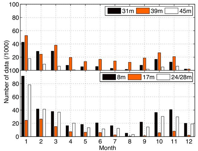
**Figure 2.** Number of data samples collected by each sonic every month from 2006 November to 2012 May. One data sample corresponds to 1 min of measurement. Top: the three upper sonics. Bottom: the three lower ones (the third was at height 28 m in 2006–2007, then at height 24 m).
