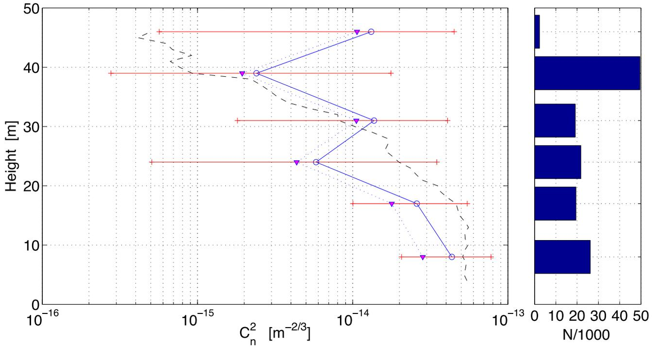
**Figure 11.**  $C_n^2$  median profile for the period April–October. Blue circles: values corrected from the bias as described in Section 4.5. Triangles: raw values. Error bars are the 50 per cent confidence interval around the blue circles. The dashed line is the median profile obtained in 2005 (March 15 to October 19) from in situ radiosoundings. The histogram on the right is the number  $N$  of valid sonic data at each altitude.
