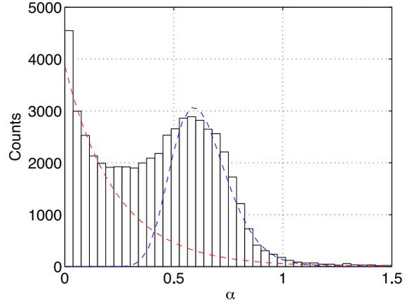
**Figure 4.** Histogram of the slopes  $\alpha$  of the structure functions  $D_T(\rho)$  of the sonic temperatures in the interval  $\rho \in [0.6 \text{ m}, 4 \text{ m}]$ . This histogram was computed from all six sonics data collected during the years 2008–2011. The dashed lines are (i) a negative exponential fit of the first part of the histogram for small values of  $\alpha$ , and (ii) a lognormal fit of the bump centred at  $\alpha = 0.6$ .
