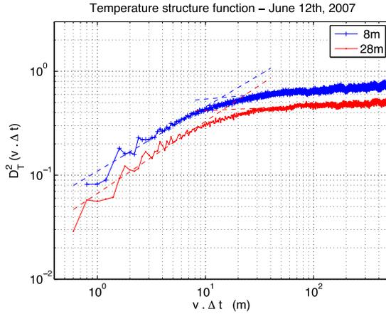
**Figure 3.** Structure functions computed from data taken on 2007 June 12. The upper curve corresponds to the 8 m sonic, and the lower one to the 28 m sonic. The dashed lines are least-squares fits of the inertial domain and on the saturation domain (large values of  $\bar{v}\Delta t$ ).
