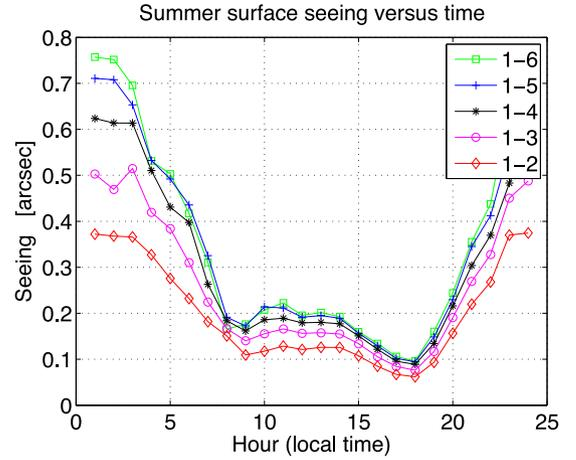
**Figure 14.** Hourly median values of the SL seeing  $\epsilon_s$  in summer (the period considered here is 2008 December where all six sonics were in operation), integrated between 8 m and the altitude of each sonic. Label such as ‘1–3’ means an integration between the first sonic ( $h = 8$  m) and the third ( $h = 24$  m).
