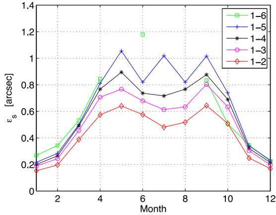
**Figure 13.** Monthly median values of the SL seeing  $\epsilon_s$  integrated between 8 m and the altitude of each sonic. Label such as ‘1–3’ means an integration between the first sonic ( $h = 8$  m) and the third ( $h = 24$  m).
