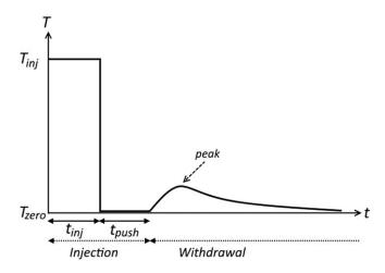
**Figure 3.** Typical push-pull breakthrough curve. The thermal tracer of temperature  $T_{inj}$  is injected during the time of injection  $t_{inj}$  and then is pushed with water of ambient temperature  $T_0$  during the push time  $t_{push}$ . Afterward, the tracer is pumped out.
