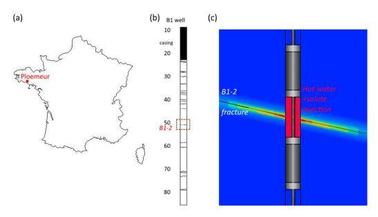
**Figure 4.** (a) Location of the Ploemeur field site, France. (b) Fracture traces measured in B1 borehole on optical and acoustic logs. Only the fractures interpreted as open from the image logs are represented (from *Le Borgne et al.* [2007]). (c) Experimental schema of a push-pull tracer test in B1-2 fracture (50.9 m depth) isolated with packers. Tracer injection as well as monitoring of temperature and conductivity were located in the middle of the double-packer system.
