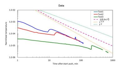
**Figure 8.** Breakthrough curves for push-pull heat tracer tests in B1 - 2 fracture. Here temperature is normalized so that its integral, over injection and pushing time, is 1.
