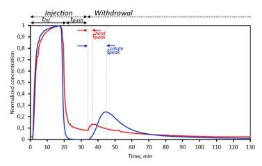
**Figure 5.** Temperature (red line) and concentration (blue line) breakthrough curves measured in between packers for Test 2. Concentrations are renormalized in order to have the same maximum value.
