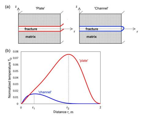
**Figure 7.** (a) Temperature distribution at the end of the injection period for (left) "plate" and for (right) "channel" (right) fracture models. (b) Temperature profiles at the fracture wall at the end of the injection period for "plate" (red) and for "channel" (blue) fracture models. Conditions of the numerical experiment correspond to the conditions of Test 1, the aperture of a = 10 mm is considered in both simulations. Temperature is normalized to the injection temperature.
