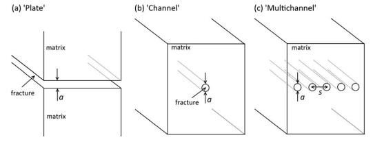
**Figure 2.** 3-D sketch for a (a) "plate" and (b) "multichannel" fracture models with parameter definitions. r direction is along the fracture hydraulic flow  $v_{fr}$ . a is the fracture aperture.  $T_0$  is the initial temperature of the rock matrix, supposed to be homogeneous and constant,  $T_{ini}$  is the fluid temperature at the fracture inlet(s).
