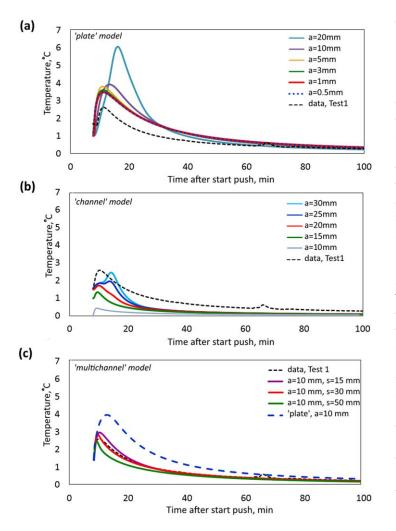
**Figure 6.** Effect of changes in fracture aperture on temperature breakthrough curve for (a) "plate" and (b) "channel" fracture models. (c) Effect of changes in fracture separation distance for "multichannel" model. Experimental data from Test 1 are given for comparison (black dashed line).
