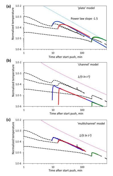
**Figure 10.** Effect of scale on temperature breakthrough curves. Comparison of experimental data (black dashed line) and results of numerical modeling (blue line—Test 1, red line—Test 2, green line—Test 3) for a (a) "plate," (b) "channel" and (c) "multichannel" fracture models.
