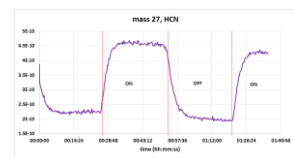
Figure 9 (top): time-monitored productions of HCN (m/z=27) showing reproducibility. The red lines show the moments the VUV source is turned ON. Figure 10 (bottom): Same but for C 2 N 2 (m/z=52)
