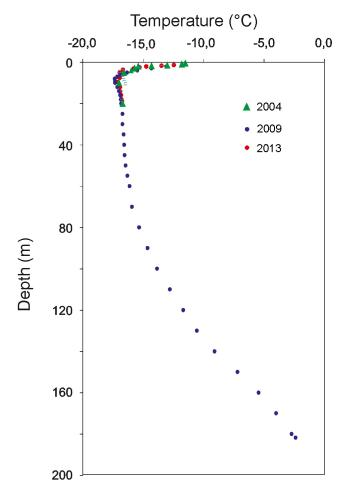
**Figure 6.** Measured temperature profiles at the western Elbrus plateau drill site for different dates: green triangles show the 22 m depth borehole drilled in 2004, blue dots show the main 2009 borehole, and red dots show the 20 m depth borehole drilled in 2013.
