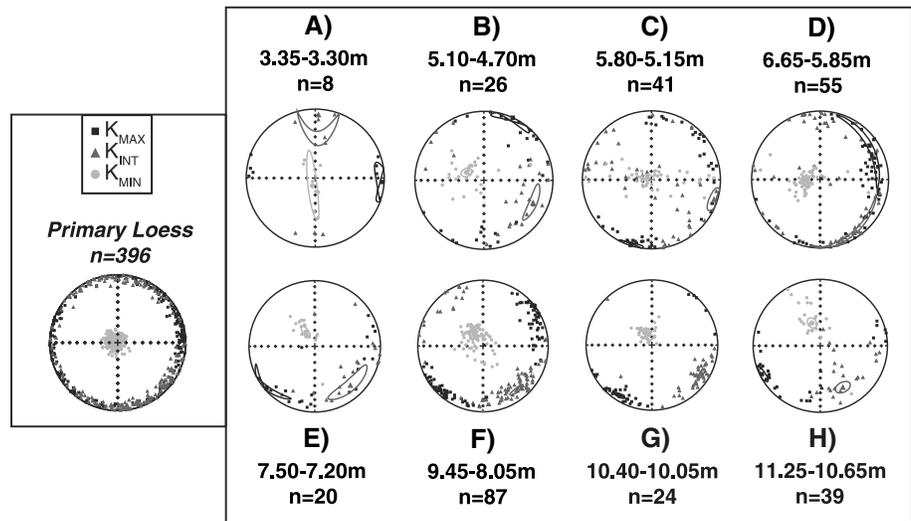
**Figure 7.** Lower hemisphere equal area stereoplots of the AMS principal axes and their 95% confidence ellipses. (left) All specimens within intervals displaying primary aeolian magnetic fabrics and (right) eight intervals interpreted as having secondary magnetic fabrics. These all show either prolate orientation distributions (A, C, and H) or oblate orientation distributions with dipping magnetic foliation planes (B, D, E, F, and G).
