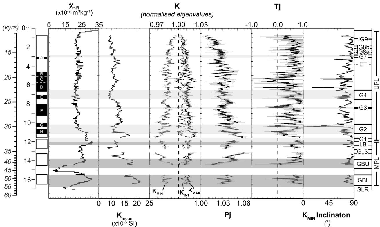
**Figure 4.** High-field magnetic susceptibility ( $\chi_{\text{hifi}}$ ), mean magnetic susceptibility ( $K_{\text{mean}}$ ), and anisotropy of magnetic susceptibility (AMS) depth-averaged parameters (error bars are the standard deviation) correlated to the stratigraphy. See Figure 1 for more information on the stratigraphic profile, and see section 2 for parameter definitions. Breaks in the data are due to unsampled depths for oriented specimens; also see section 2 for explanation.
