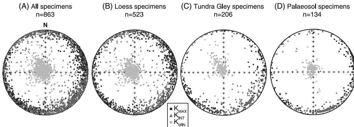
**Figure 6.** Lower hemisphere equal area stereoplots of (a) all Nussloch P8 specimens, (b) loess, (c) main tundra gleys (G2–G7; G1 and G<sub>M</sub>3 were not sampled), and (d) palaeosols (GBL, GBU, and LB). Tensor mean values are listed in Table 2.
