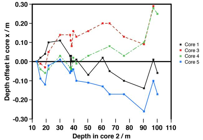
**Figure 5.** Depth offset of 18 common and securely identified volcanic events in cores 1, 3, 4 and 5 relative to core 2. To overcome offset due to the drilling process and poor core quality in the first meters, UE 1809 (depth: ca. 13 m) is taken as the origin and horizon reference.
