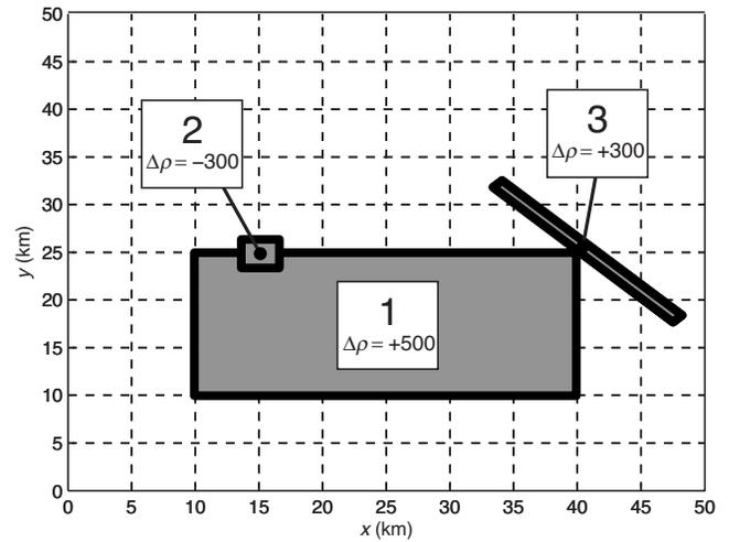
Figure 1. Projection, onto the  $(x,y)$ -plane, of the three blocks described in Table 1. Density contrasts  $\Delta\rho$  are in kilograms per cubic meter ( $\text{kg}/\text{m}^3$ ).
