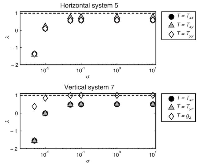
Figure 4. Variations of  $\lambda$  according to the logarithm of the noise standard deviation  $\sigma$ , in Eötvös for the gravity gradients and in milligals for  $g_z$ , on a regular square grid with a step of 200 m.
