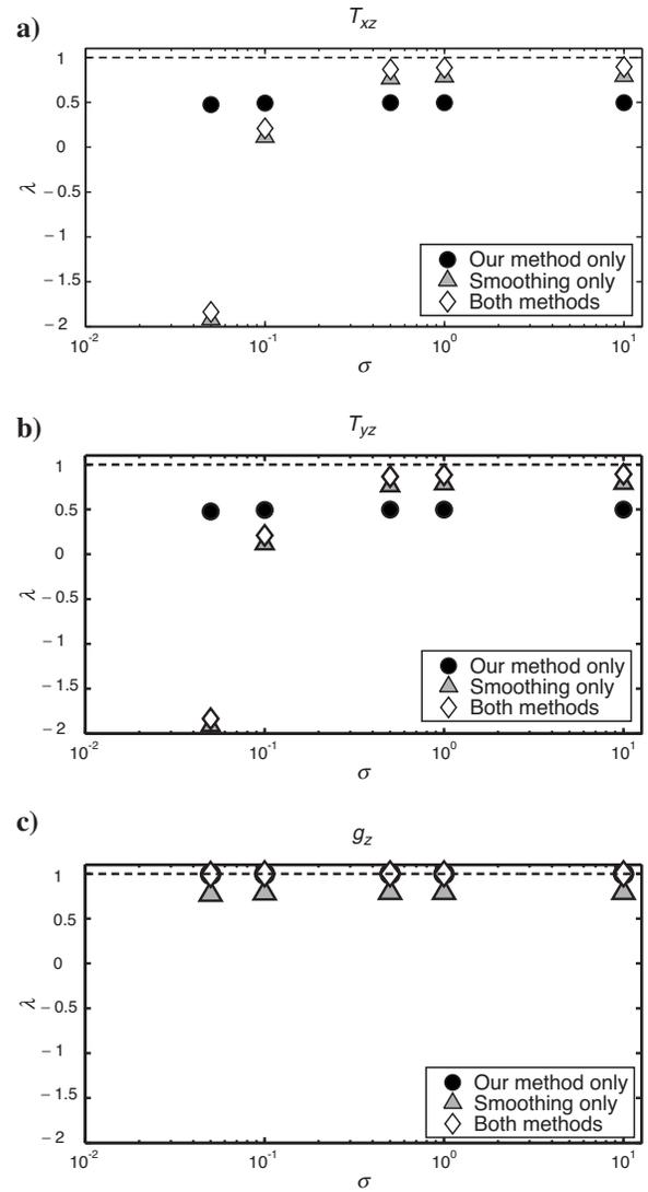
Figure 6. Comparison, on a regular square grid with a step of 200 m, between the impact of Gaussian smoothing in a  $3 \times 3$  point window and our noise-reduction method for (a) the tensor component  $T_{xz}$ , (b) the tensor component  $T_{yz}$ , and (c) the component  $g_z$  involved in vertical system 7.
