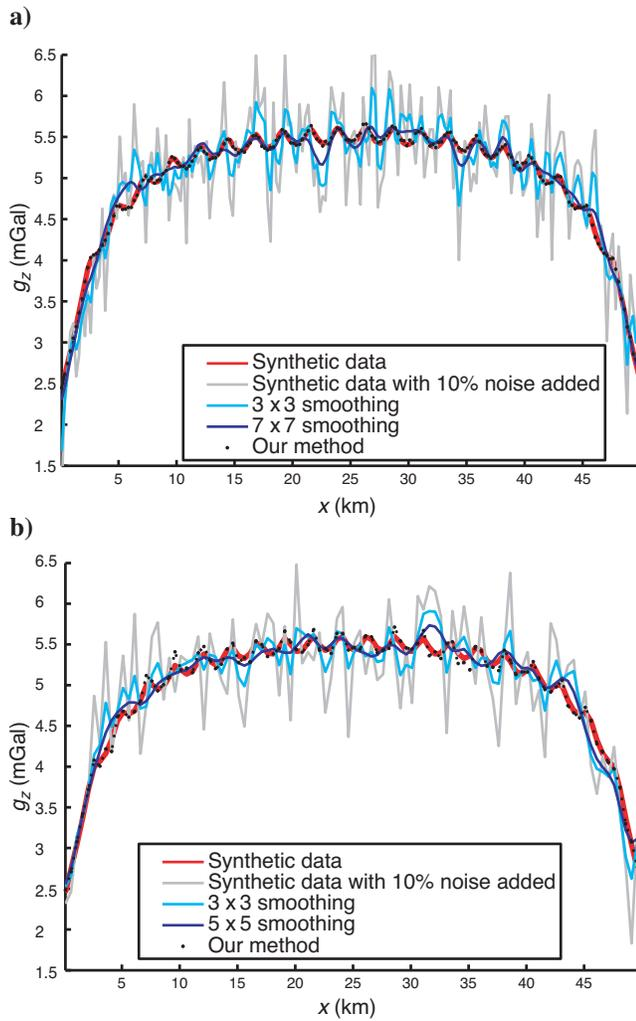
Figure 8. Comparison along a profile for a grid step of (a)  $250\text{ m}$  and (b)  $500\text{ m}$  between the noise-reduction results of our method and Gaussian smoothing with varying window size, applied on  $g_z$ . In the background, gray represents the anomaly with  $10\%$  noise added, red the original anomaly, dotted black our result, and dark and light blue the results of Gaussian smoothing.
