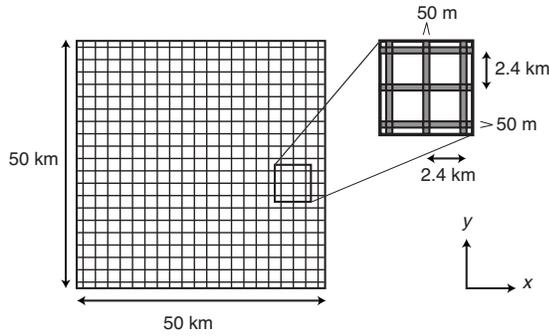
Figure 7. Projection onto the  $(x,y)$ -plane of the structure used to show how our method handles small wavelengths. The structure is made of 40 identical rectangular prisms arranged in an orthogonal lattice, each prism having  $(x,y)$ -dimensions of  $50\text{ m} \times 50\text{ m}$ . The depth to the top sides of the prism is  $30\text{ m}$ . The depth to the bottom is  $10,000\text{ m}$ . The density contrast is  $1000\text{ kg/m}^3$ .
