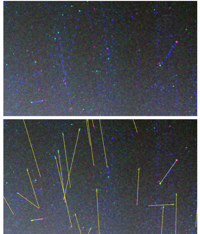
Figure 3. RGB composite of the 20 movie frames. The blue channel shows the maximum stack of all 20 movie frames (cf. Fig. 2). The red and green channels show the first and last image of the movie sequence, respectively. Both panels show the same image section and have an angular size of 0^\circ 5' \times 0^\circ 3' . The lower panel in addition shows the identified tracks as yellow arrows.
