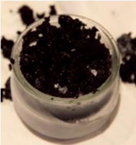
Figure 3. The cometary analogue sample in a glass container.
