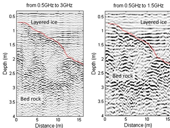
**Fig. 6.** Examples of radargrams obtained by WISDOM in the Dachstein ice cave [51], Austria (with the whole frequency bandwidth on the left and with only 1 GHz of bandwidth on the right). The layered ice is visible on the upper right part of the figures. The red line highlights the transition with the bedrock beneath the ice.
