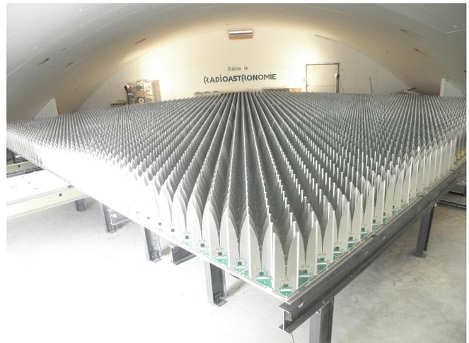
**Fig. 1.** EMBRACE@Nançay is composed of 4608 Vivaldi antenna elements separated from each other by 12.5 cm, making it a dense array for frequencies above 1200 MHz. EMBRACE@Nançay measures 8.42 m × 8.42 m for a total area of 70.8 m<sup>2</sup>.
