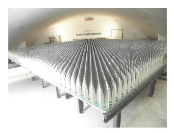
Fig. 1. EMBRACE@Nançay is composed of 4608 Vivaldi antenna elements separated from each other by 12.5 cm, making it a dense array for frequencies above 1200 MHz. EMBRACE@Nançay measures  $8.42 \text{ m} \times 8.42 \text{ m}$  for a total area of  $70.8 \text{ m}^2$ .
