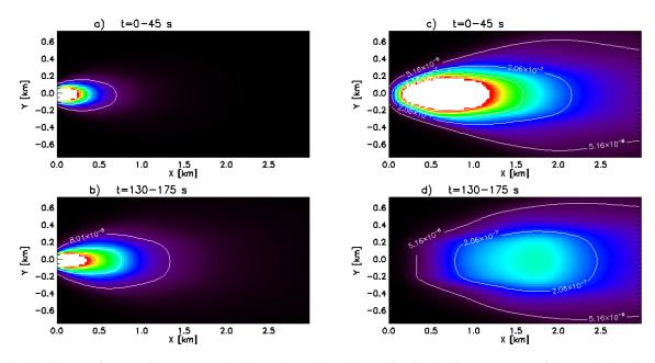
Fig. 12. Simulated images integrated between t = 0-45 s and t = 130-175 s (to simulate the long exposures of the UV-375 nm images) for two different source functions. In the *left panels* **a**) and **b**) the production rate is kept constant during the whole simulation, on the *right* (**c**) and **d**)) the production was stopped at t = 5 s. In this case the moving dust cloud has detached from the source at t = 130-175 s and a rather flat brightness distribution can be seen.
