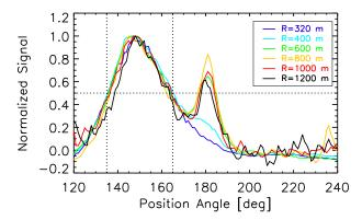
**Fig. 5.** Normalized angular radiance distribution as a function of position angle on circles around the estimated source point. The angular profile resembles a Gaussian and for distances between 300 m and 1000 m from the source the FWHM of the jet is approximately constant at about  $30^{\circ}$ .
