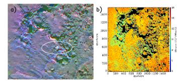
Fig. 8. Detected outburst region, a) decorrelation stretched image, b) spectral slope, the white cross indicates the best estimate of the jet source point and the ellipse provides the  $2\sigma$  uncertainty.
