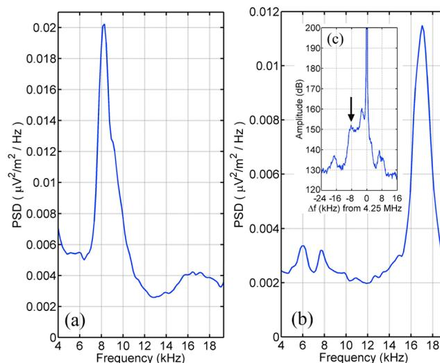
**Figure 3.** Power spectral density versus frequency measured on 16 October 2009 (Figure 2a) and on 2 October 2010 (Figure 2b), obtained from a 2 s average of the Figure 2 observations near the closest approach of the MZ. SEE spectrum observed on the ground at HAARP on 2 October 2010 (Figure 3c);  $\Delta f$  is the observed frequency relative to the pump frequency.
