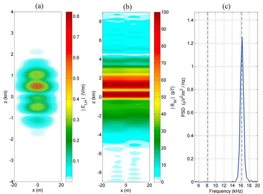
**Figure 6.** Simulation results showing generation of mode-converted whistler waves with frequency equal to the LH second harmonic: (a) The magnitude of the LH electric field in V/m, (b) magnitude of the whistler magnetic field in picotesla, and (c) spectrum of the y component whistler electric field; the vertical lines in Figure 6c represent the LH frequency and its second harmonic.
