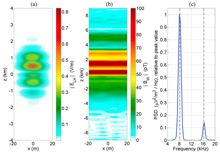
**Figure 5.** Simulation results showing generation of mode-converted whistler waves with frequencies at the LH frequency and its second harmonic: (a) the magnitude of the LH electric field in V/m, (b) magnitude of the whistler magnetic field in picotesla, and (c) spectrum of the y component whistler electric field, relative to the peak value; the vertical lines in Figure 5c represent the LH frequency and its second harmonic.
