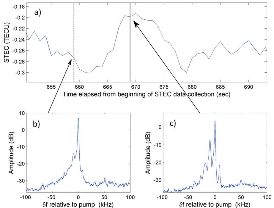
**Figure 4.** (a) Measurements of STEC during an HF heating experiment; variation in STEC has a timescale of several seconds. (b) Simultaneously, SEE was measured 20 ms after the start of heating, already showing signs of DM. (c) SEE after 10 s of heating shows well-developed DM, along with 2DM and 3DM.
