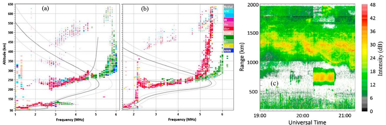
**Figure 1.** Ionograms (a) during Experiment 1 and (b) during Experiment 2 showing a smooth ionosphere with sporadic E layer present, as well as Kodiak radar observations (c) during Experiment 1 showing strong reflections (given in decibel) during the time of heating (20:15–20:45 UT) in the range 700–800 km.
