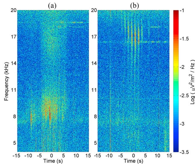
**Figure 2.** Spectrogram seen by DEMETER (a) during Experiment 1 on 16 October 2009 in which HAARP used CW heating and (b) during Experiment 2 on 2 October 2010 in which HAARP used 0.7 Hz square pulse modulated heating. In both cases time = 0 corresponds to the closest approach of DEMETER to the HAARP magnetic zenith.
