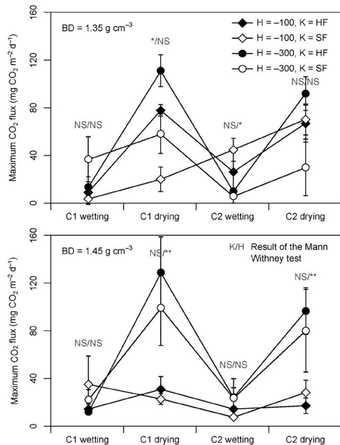
**Fig. 6.** Maximum carbon dioxide fluxes recorded during the four successive hydric steps (C1: first wetting-drying cycle, C2: second wetting-drying cycle) for soil samples of bulk density BD = 1.35 and 1.45 g cm<sup>-3</sup> (H: pressure head applied, in hPa, K: saturated hydraulic conductivity of the porous plate, HF: high flow, SF: standard flow). Error bars represent standard error of the mean (n = 3).
