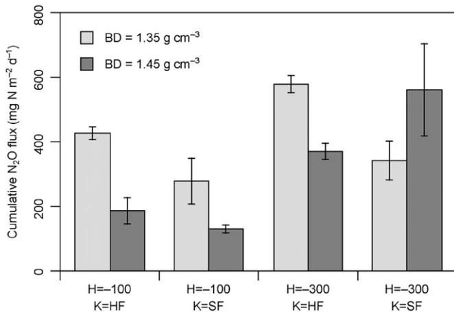
**Fig. 5.** Cumulative nitrous oxide fluxes at the end of the second wetting-drying cycle for samples of bulk density  $BD = 1.35$  and  $1.45 \text{ g cm}^{-3}$  (H: pressure head applied, in hPa, K: saturated hydraulic conductivity of the porous plate, HF: high flow, SF: standard flow). Error bars represent standard error of the mean ( $n = 3$ ).
