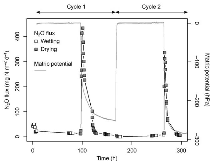
**Fig. 2.** Evolution with time of the nitrous oxide fluxes and matric potential of a sample of bulk density  $BD = 1.45 \text{ g cm}^{-3}$ , pressure head applied  $H = -300 \text{ hPa}$ , and a high flow porous plate, during two wetting-drying cycles. For the sake of readability, the measurement points are linearly interpolated.
