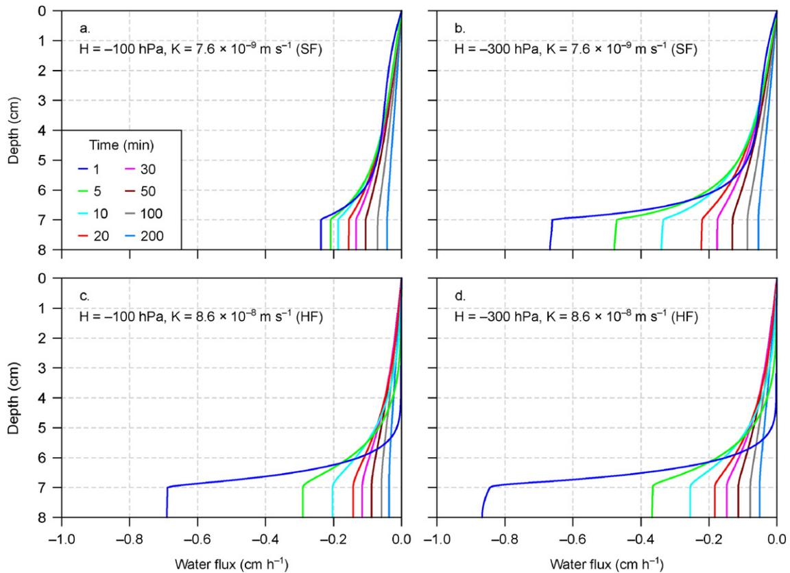
**Fig. 7.** Simulated profiles of water flux with time just after the beginning of the soil drying of a sample of bulk density  $BD = 1.35 \text{ g cm}^{-3}$  (H: pressure head applied, K: saturated hydraulic conductivity of the porous plate). Because a drying phase is simulated, the water flux is negative.
