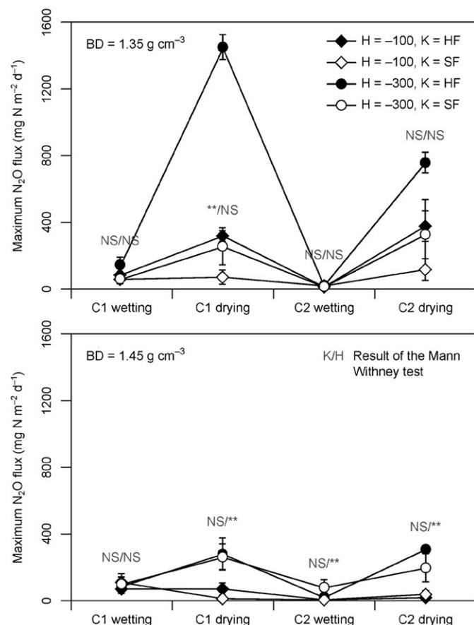
**Fig. 3.** Maximum nitrous oxide fluxes recorded during the four successive hydric steps (C1: first wetting-drying cycle, C2: second wetting-drying cycle) for soil samples of bulk density BD = 1.35 and 1.45 g cm<sup>-3</sup> (H: pressure head applied, in hPa, K: saturated hydraulic conductivity of the porous plate, HF: high flow, SF: standard flow). Error bars represent standard error of the mean ( $n = 3$ ).
