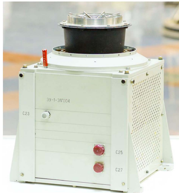
Figure 2. One of two heads of SCA-1. The analyzer is located on the top of electronics box.
