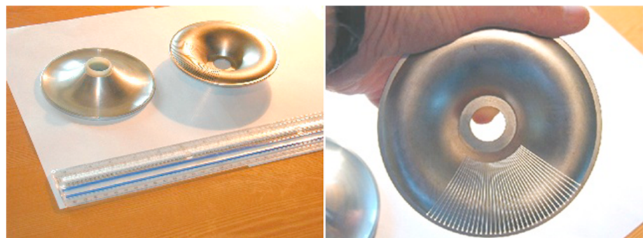
Figure 13. (left) Electrostatic mirror electrodes and (right) external electrode representing made of single appropriate shaped detail with radial slits.
