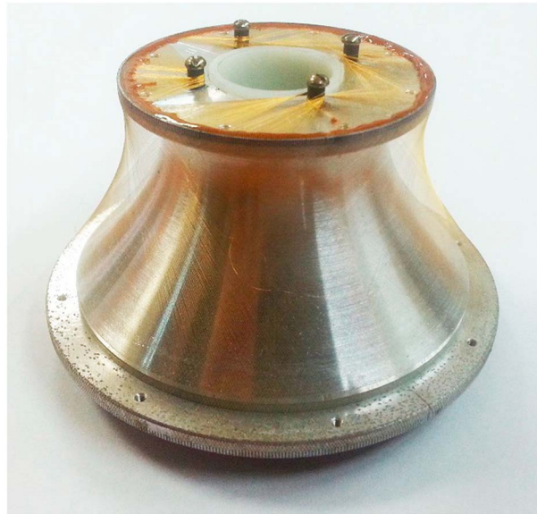
Figure 6. Mirror for Fonema/Mars-96 energy-mass analyzer providing wide-angle acceptance angles in hemisphere for 18 narrow-angle Thomson parabola analyzers. External transparent electrode is a parabolic hyperboloid made of thin wires. Design of external electrode was inspired by Shukhov’s tower by famous Russian engineer, architect, and scientist Vladimir Shukhov.
