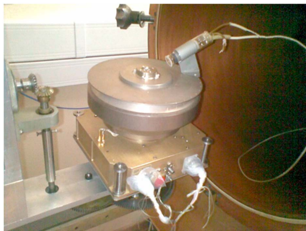
Figure 17. DI-Aries for Phobos-Soil mission in vacuum chamber. Preparing to test of the response to UV.
