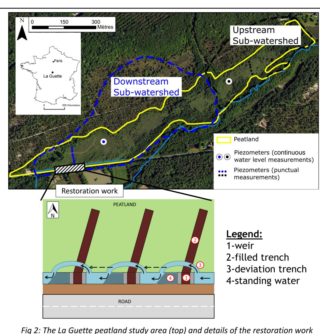
Fig 2: The La Guette peatland study area (top) and details of the restoration work (bottom)
