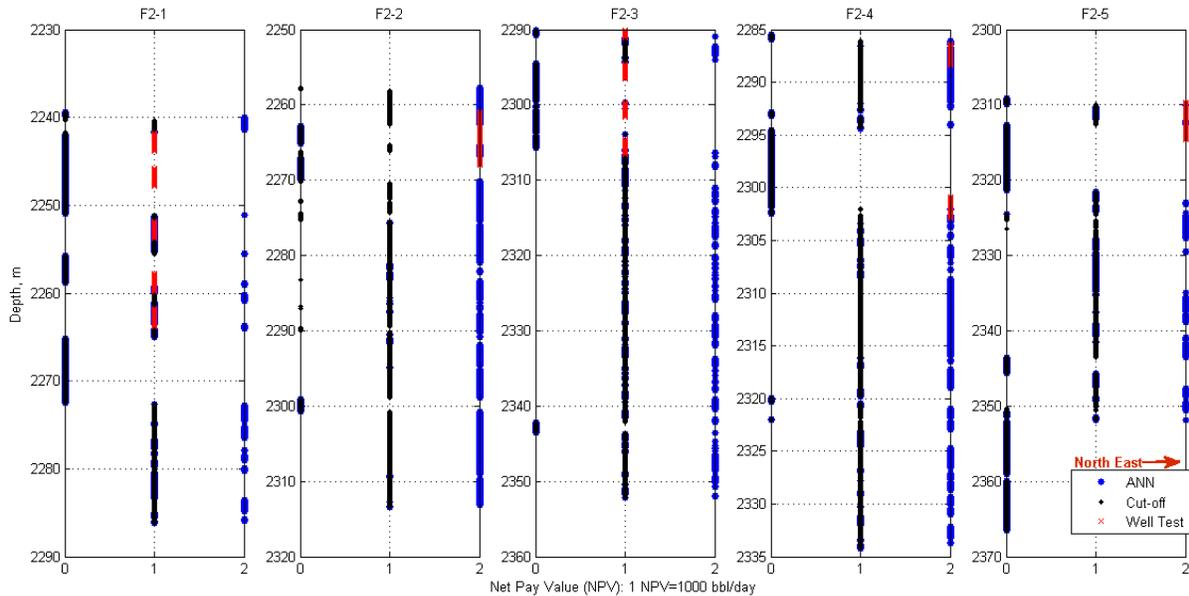
Figure 7 Net pay determination in five wells of the Second Field, studying Sandy Burgan reservoir. The vertical axe is depth versus the horizontal axe of Net Pay Value.
