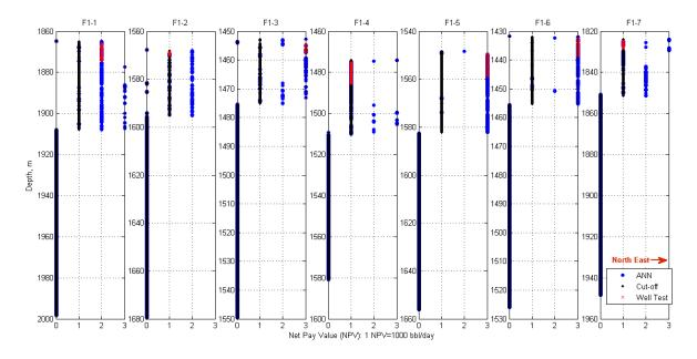
Figure 6 Net pay determination in seven wells of the First Field, studying carbonate Mishrif reservoir. The vertical axe is depth versus the horizontal axe of Net Pay Value.
