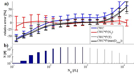
**Figure 3.** (a) Relative errors of  $\overline{\text{CWC}}$  with respect to  $\text{CWC}_{\text{IKP}}$  (as defined in Table 1) as a function of total PSD number concentration  $N_T$ . The errors are presented with and without the three suggested correction functions for  $\overline{\text{CWC}}$ . (b) Number of 5 s data points used for the statistics on the y axis as a function of  $N_T$  intervals.
