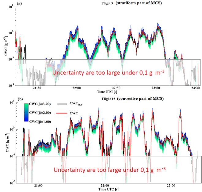
**Figure 1.** Condensed water content (CWC) as a function of time for two HAIC/HIWC flights during the Darwin 2014 flight campaign. In black is  $CWC_{IKP}$ ; in red is the average  $\overline{CWC}$  deduced from all possible simulations (varying  $\beta$  and constraining  $\alpha$ ) of the measured  $Z$ . Blue-to-green colour band shows  $CWC(\beta_i)$  calculations when  $\beta$  varies from 1 (blue) to 3 (green). (a) Results for flight 9; (b) results for flight 12.
