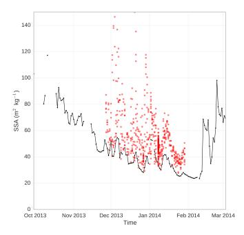
**Figure 15.** Time series of daily mean SSA averaged for the two heads of Autosolexs (black line) and manual measurements taken using ASSSAP (red dots). Both instruments have different vertical sensitivity as illustrated in Fig. 1.
