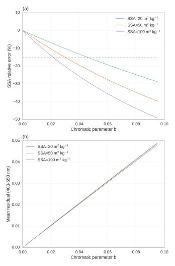
**Figure 4.** (a) Theoretical calculation of the relative error in SSA due to the chromatic aberration of the spectrometer as a function of the parameter *b* defined in Eq. (8) for SZA =  $60^{\circ}$ . The dashed line shows the 15 % target accuracy discussed in the paper. (b) Relationship between *b* and the residual between the observed and estimated albedo averaged over the range 400–550 nm.
