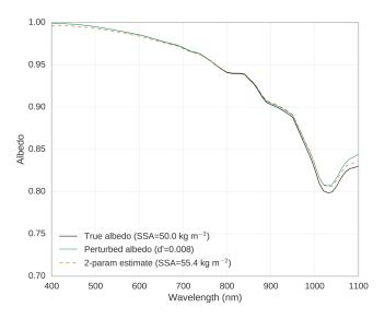
**Figure 11.** Simulations of albedo spectrum for a SZA =  $60^{\circ}$ . A perfect albedo spectrum for an homogeneous snowpack with SSA of  $50 \text{ m}^2 \text{ kg}^{-1}$  (black) is perturbed (green) by adding an offset of d' = 0.8% of the maximum incident irradiance to the incident and reflected irradiance. It is used as an observation to estimate SSA using the range 700–1050 nm. The estimated spectrum is shown in orange (long dash).
