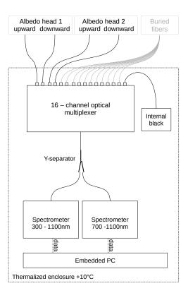
**Figure 6.** Principle of Autosolexs. The dotted rectangle represents the thermalized container that is buried in the snow. The plain curved lines represent fiber optics, the fibers buried in snow (gray) are not used in the present study.
