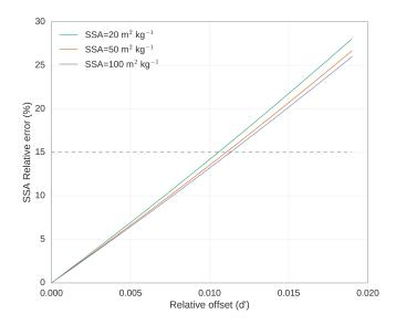
**Figure 2.** Theoretical calculation of the relative error in SSA due to an offset in the incident and reflectance spectra for SZA =  $60^{\circ}$ . The dashed line shows the 15 % target accuracy discussed in the paper.
