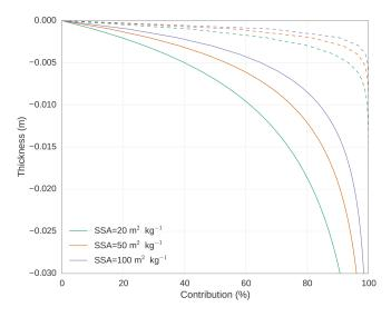
**Figure 1.** Contribution of the uppermost layer of a semi-infinite snowpack to the albedo averaged over the range 700–1050 nm (plain line) and at 1310 nm (dash line) as a function of the layer thickness.
