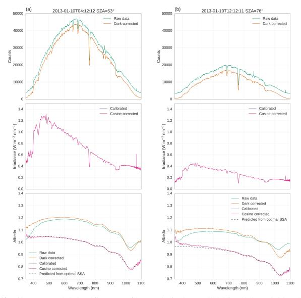
**Figure 10.** Incident spectrum and albedo at different stages of the processing for 10 January 2013 (left) at 12:12 LT and (right) at 20:12 LT. Raw data (green) are first corrected for the dark current and stray light (orange) then calibrated (violet) and last corrected for imperfect collectors (pink). The theoretical spectrum that fits the fully corrected spectrum (pink) is shown in black.
