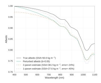
**Figure 3.** Simulations of albedo spectrum for SZA =  $60^{\circ}$ . A perfect albedo spectrum for an homogeneous snowpack with SSA of  $50 \text{ m}^2 \text{ kg}^{-1}$  (black) is perturbed by a factor linearly decreasing from 1 at 400 nm to 1 - b at 1100 nm with b = 5% (green) and used as an observation to estimate SSA with the one-parameter (violet thin dash) and two-parameter models (orange, long dash). Estimated values are shown in the legend along with the relative error.
