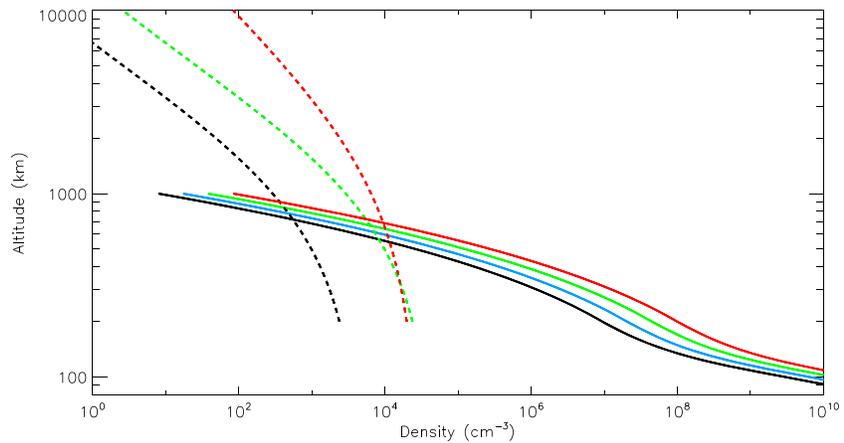
**Figure 1.** Examples of cold oxygen density profiles (solid lines) and hot oxygen density profile (dashed lines) used as input of the radiative transfer model. The cold oxygen profile has been derived using an exospheric temperature of 300 K, while different scale heights (~300 km for the black and green profiles and ~1200 km for the red profile) are used to simulate the hot oxygen corona.
