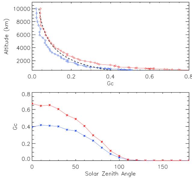
**Figure 4.** (top)  $G_c$  factor variations with altitudes for two different cold oxygen density profiles (see Figure 1) at SZA = 30°. The black dashed line represents the expected asymptotic variation in  $1/r^2$ . (bottom)  $G_c$  variations with SZA for the same density profiles near 750 km.
