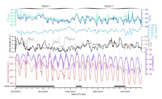
**Figure 8.** Hourly average  $\delta D$  (‰) in dark blue, hourly average  $\delta^{18}O$  (‰) in green, d-excess (‰) smoothed on a 3 h span in light blue and hourly average of the specific humidity (ppmv) in red, measured by the Picarro during the campaign; comparison with 3 m temperature (purple, °C), difference between ground and 3 m temperature (purple shade, °C), wind direction (grey dots, °) and speed (black line).
