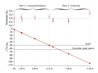
**Figure 6.** Isotopic composition measured by liquid injection in the Picarro L2140i for different samples prepared by dilution of EPB with "almost pure" water: the red dots are the measurements, the red line is the calculated isotopic composition and the red squares for residuals are the difference between the measurements and the theoretical composition.
