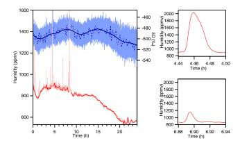
**Figure 5.** Left: example of raw data measured by the Picarro. Humidity (light red, ppmv) and  $\delta D$  (light blue, %), data averaged over 10 min for humidity (red, ppmv) and for  $\delta D$  (dashed line blue, %) and over 1 h for  $\delta D$  (dark blue, %). Right: zoom on two "precipitation events" identified in the humidity signal of the Picarro (top, snow flake; bottom, diamond dust).
