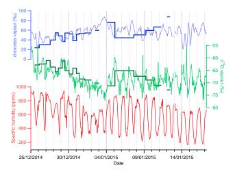
**Figure 7.** Hourly average  $\delta^{18}O$  (‰) in green, raw d-excess (‰) in light blue (d-excess smoothed on a 3 h span in thick blue) and hourly average of the specific humidity (ppmv) in red during the campaign 2014/2015. Measurements by the Picarro are displayed as the thin light lines and measurements performed in the laboratory from the cold trap samples are displayed as dark bars.
