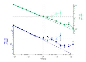
**Figure 3.** Allan variance plots for laboratory long-term standard measurement (dark squares) and for field long-term standard measurement (light circles) for  $\delta D$  (Top, green) and for  $\delta^{18}O$  (bottom, blue). Dash lines correspond to the quantum limit on  $N^{-1/2}$  for each composition.
