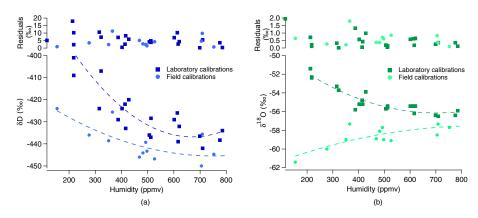
**Figure 4.** Measured isotopic composition for (a)  $\delta D$  and (b)  $\delta^{18}O$  using the PICARRO spectrometer for a fixed humidity: light circles are field calibration points, dark squares are laboratory calibration points, the dashed lines are the fit with a quadratic function and at the top are the residuals compared to the fit for the entire series.
