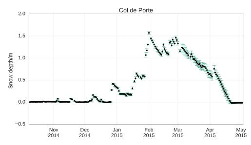
Figure 3. Evolution of the mean (black) and standard deviation (green) of the snow depth at Col de Porte over the winter season 2014–2015 measured by the RLS.
