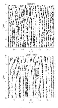
**Figure 10.** Zoomed image of the scans at Dome C and Col de Porte acquired 15 February 2015. Each point shown in the (x, y) plan is an individual measurement of the laser meter.
