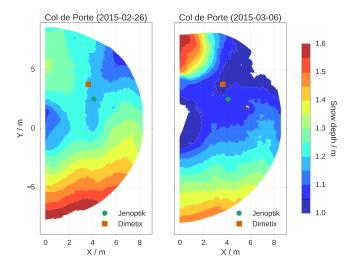
**Figure 8.** Two snow depth maps acquired at Col de Porte 26 February 2015 when the snow depth reaches its maximum and 6 March 2015 after a wind slab appeared in the northern corner (x = 0; y = 6 m). North is approximately in the *y*-axis direction. The square and round symbols represent the footprint of the SPICE sensors at the beginning of the season.
