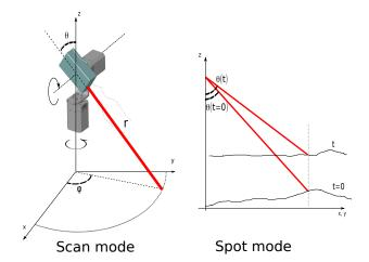
**Figure 1.** Principle of the scan mode and spot mode of the Rugged Laser Scan (RLS). The zenith angle  $\theta$  and azimuth angle  $\phi$  determine the orientation of the laser meter which measures the range *r*.
