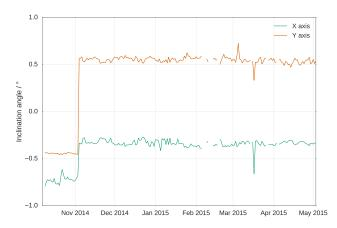
**Figure 6.** Evolution of the inclination of the laser over the season at Col de Porte.
