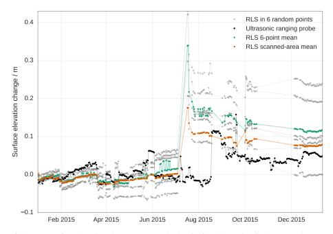
**Figure 12.** Evolution of the snow surface elevation change at Dome C taken in 6 random points in the scanned area (gray), on average over the 6 points (green), on average over the scanned area (orange) and measured by a nearby ultrasonic ranging probe (black).
