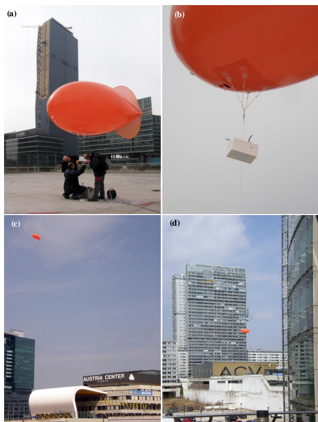
Figure 4. Pictures of the LOAC operations below a 6\text{ m}^3 tethered balloon at the Austria Center in Vienna during the 2013 European General Assembly. From left to right and top to bottom: (a) preparation of the launch with a view towards the south on a tower under final stage of construction in the back; (b) view from below of LOAC in flight with its sampling inlet pointing upward; (c) view from the S of the balloon over the conference centre; (d) view from the south-west of the environment of the launch site including leaving and office tower blocks and an open air car park.
