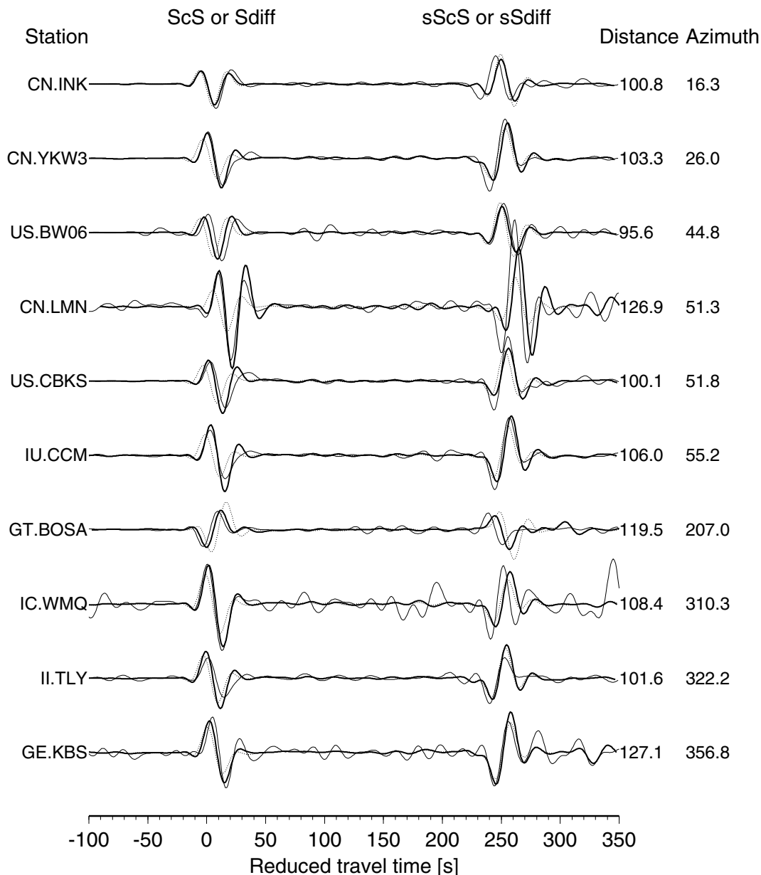
Figure 11. Comparison between data (thin line), synthetics in PREM (dotted line) and synthetics in SAW24B16 + PREM (bold line).
