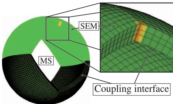
**Figure 2.** Left: global view of the model where two regions have been removed for sake of visibility. The SEM mesh is drawn only for two regions. Right: zoom on the plume inclusion area. The colors indicate the S wave velocity contrast with respect to the modified PREM model. On this figure, the plume radius is of 250 km and the maximum S-velocity contrast is 4.5%.
