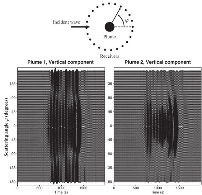
**Figure 3.** Vertical component of the scattered field, as a function of the scattering angle  $\varphi$ , as detailed by the top sketch, for two plume-like cylindrical structures of 100 km radius (left) and 250 km radius (right). The forward scattering pattern increases with the plume radius. The maximum scattering amplitude is related to surface waves.
