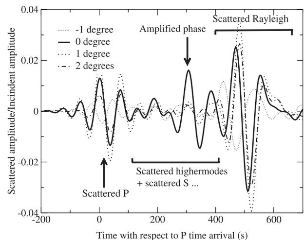
**Figure 4.** Vertical component of the scattered field for the small plume (plume 1), at four angular distances along the source-plume great circle:  $-1$ ,  $0$ ,  $1$  and  $2$  degrees from the plume. The arrow indicates a scattered amplified phase for the receiver on top of the plume.
