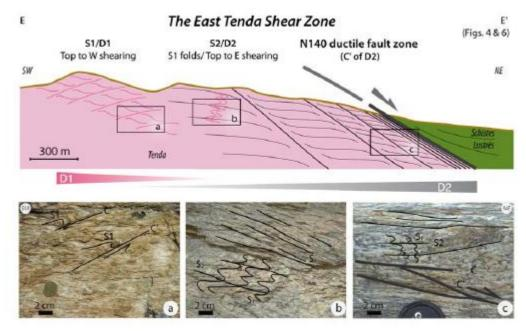
Figure 5/ N140° ductile fault zones: SW-NE cross-section in the East Tenda Shear Zone (ETSZ, location EE' in Figs. 4 and 6) showing the superposition of two deformation events (D1 and D2). A-B-C/ Outcrop photographs of the main types of structures. See locations on the cross-section.
