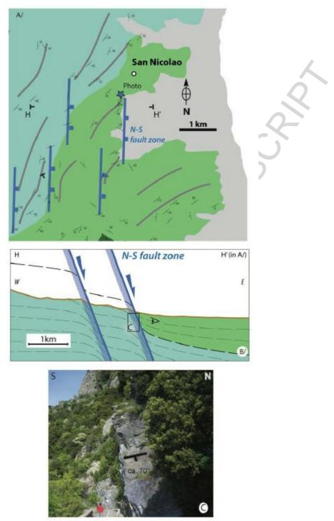
Figure 8/ N-S fault zones in the Schistes Lustrés in the vicinity of San Nicolao (See location in Fig. 3). A/ Detailed structural map illustrating the change in foliation trends. B/ E-W crosssection (location HH' in A/) showing the deformation zone (flexure in light blue) associated with N-S fault zones (see text for further details). C/ outcrop photographs of steeply dipping foliations (location in B/).
