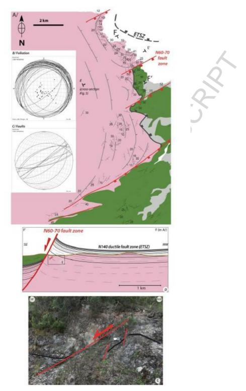
Figure 6/ N60°-70° fault zones in the Tenda massif (location in Fig. 4): A/ Detailed tectonic map of the ETSZ with N60°-70° trending normal fault zones and locations of cross-sections EE' (shown in Fig. 5) and FF' (shown in D/). B-C/ Stereoplots of foliations and faults measurements. D/ NNW-SSE cross-section (location FF' in A/) showing the rework of the ETSZ (N140 fault zone) by N60-70 fault zones. E/ Outcrop photographs (location in D/).
