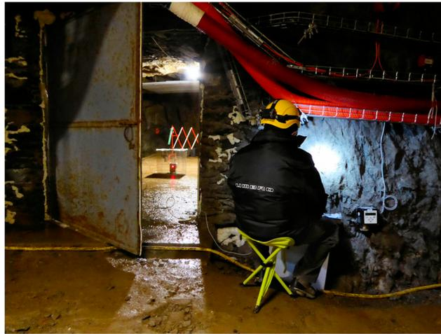
**Figure 11.** Conductivity sensors tests in the inner room of the Roselend tunnel. The metal door used to isolate the inner room from the tunnel is open half-way. The Sensor is set in the middle of the inner room. The operator is sitting outside the inner room, in the tunnel. Surfaces appear shiny due to moisture condensation.
