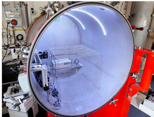
**Figure 4.** Setting of the conductivity sensors tests in the BACCARA chamber.
