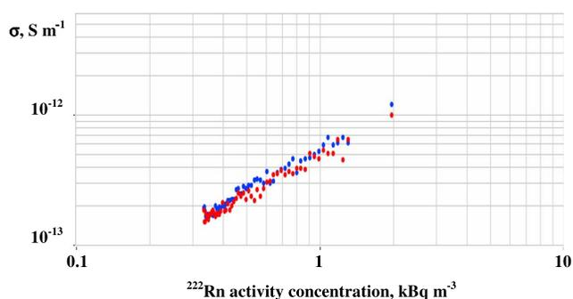
**Figure 15.** Electric conductivity ( $\sigma$ ) of moist air, measured by the conductivity sensors in the inner room of the Roselend tunnel, versus  $^{222}\text{Rn}$  activity concentration, at the pressure of 845 mbar and air relative humidity of 97%. Red and blue dots indicate the electric conductivity carried by the positive and negative ions, respectively.
