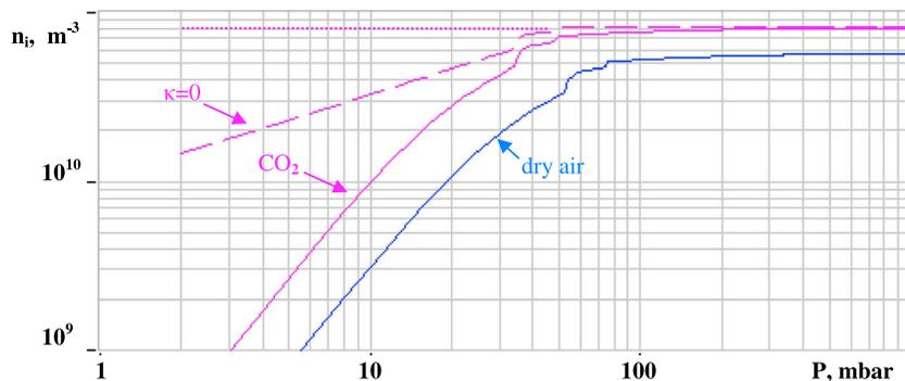
**Figure 8.** Ion density ( $n_i$ ) versus gas pressure ( $P$ ) deduced from the electric conductivity represented in Figure 7. Descriptions of different types of lines and their colors are identical to those of Figure 7.
