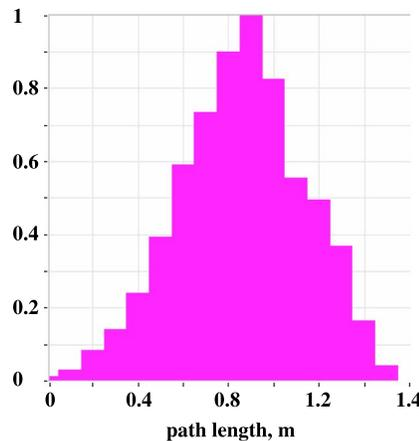
**Figure 3.** Probability distribution of 6MeV-alpha path length in the BACCARA chamber (cylinder with a diameter of 1 m and a length of 1.3 m) at 6mbar pressure. Mean value is estimated to be  $\sim 0.86\text{ m}$ .
