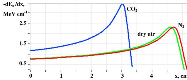
**Figure 2.** Energy loss rate of 6MeV-alpha particle versus distance along its path in dry air (green line), nitrogen (red line), and carbon dioxide (blue line) at  $P=975\text{mbar}$  and  $T=25^\circ\text{C}$ .
