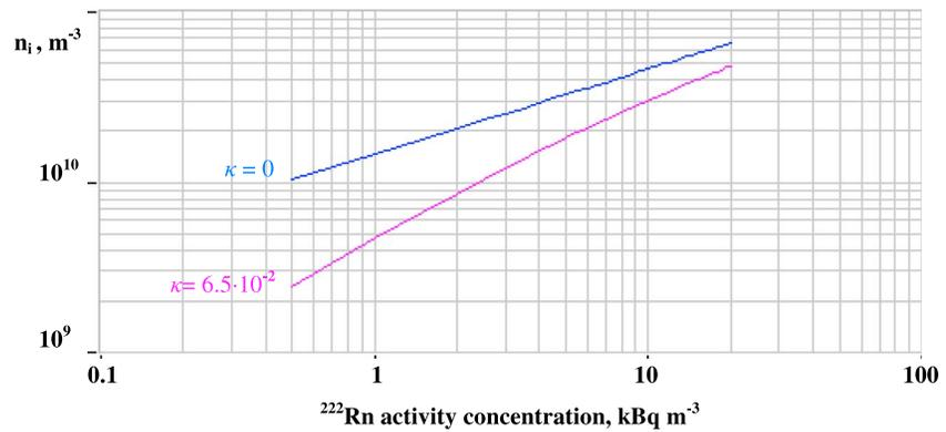
**Figure 6.** (mauve line) Ion density which corresponds to the air electric conductivity shown by mauve line in Figure 5. (blue line) Ion density calculated using the same parameters as for the mauve line but with the assumption that there is no ion sink on the chamber walls; i.e.,  $\kappa=0$ .
