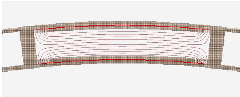
Figure 8. Cut view of a single sector of the analyzer showing the electrostatic potential map. Separators are grounded. A transition region between the separators and the main part of the high-voltage biased electrodes is defined where the potential varies linearly.
