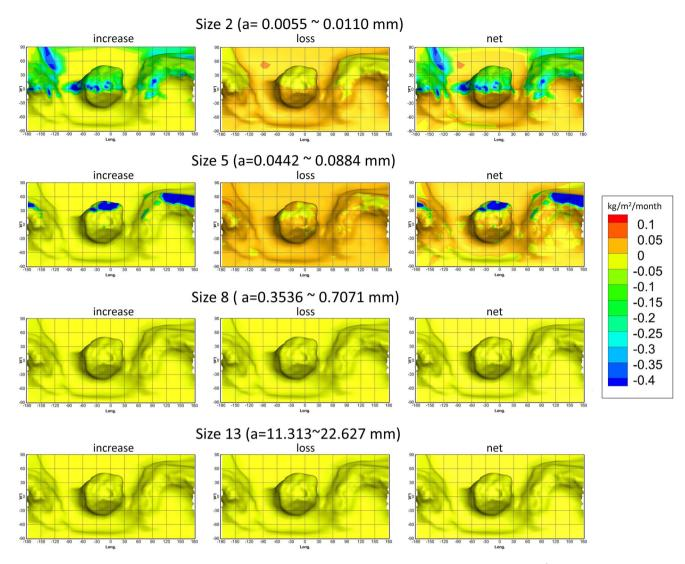
Figure 9. Examples of the spatial distributions of the mass-loss rate, mass influx and net mass change rate (in unit of kg  $m^{-2}$  per month) of several selected dust sizes in 2015 January.
