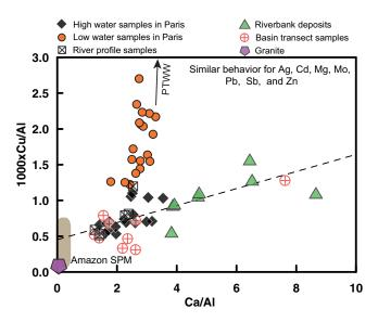
**Figure 7.** Cu/Al versus Ca/Al for all sediments, anthropogenic, and 2 bedrock samples of the Seine basin. Gray areas represent the range (average  $\pm$  2SD) of Cu/Al and Ca/Al ratios in Amazon River SPM [data from *Bouchez et al.*, 2011a]. The riverbank deposit RBD9 was not included because of its extremely high and most likely unrepresentative carbonate (shell) content.
