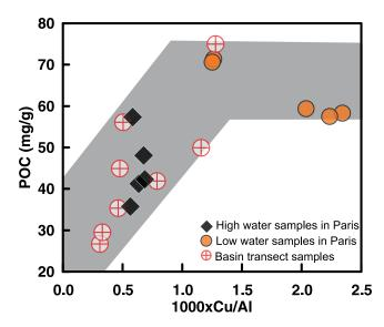
**Figure 10.** Particulate organic carbon (POC) content versus Cu/Al ratio. The increase of Cu/Al ratio with POC implies that Cu is mostly associated with organic matter in flood samples, while for the low water stage samples the different trend may indicate other major Cu carriers such as sulfides. Element/Al ratios for Bi, Cd, Cr, Cu, Fe, Mg, Mn, Mo, Pb, Sb, Sn, W, and Zn show similar relationships with POC.
