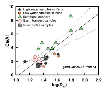
**Figure 4.** Relationship between sediment chemical compositions, as indexed by the Ca/Al ratio, and grain size median distribution ( $D_{50}$ ) measured for some samples. High Ca/Al ratios are characteristic of carbonate-rich, coarse sediment such as riverbank deposits (RBD, excluding RBD9), while clay enrichment (Al enrichment) is observed in suspended particulate matter (SPM).
