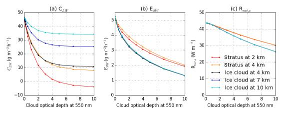
**Figure 10.** Sensitivity of  $C_{LW}$  (a),  $E_{SW}$  (b) and  $R_{net,s}$  (c) (defined in Sect. 2.1) to the altitude, type and visible optical depth of a cloud appearing above the fog. All other input data are kept constant at the values for 13 December 2015 at 10 UTC (the same time as in Fig. 9). Solar zenith angle is 75.7°.
