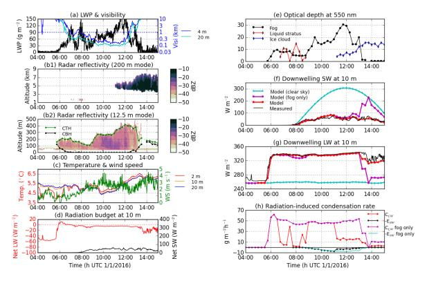
**Figure 7.** Case study of the fog event on 1 January 2016, when clouds appeared above the fog. Panels are the same as in Fig. 3, with a few additions. In **(b)**, there are two panels, the upper one showing the reflectivity from the 200 m mode of the radar and the lower one that of the 12.5 m mode. In **(e)**, the optical depths of the cloud layers above the fog are also indicated, and in **(f-h)** the results obtained when including only the fog (and not the higher clouds) have been added.
