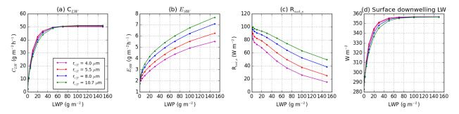
**Figure 8.** Dependency of  $C_{LW}$  (a),  $E_{SW}$  (b),  $R_{net,s}$  (c) (defined in Sect. 2.1), and the downwelling LW flux at the surface (d) on the fog LWP and effective radius. All other input data are fixed to the values of 27 October 2014 at 08:30 UTC: the fog is 100 m thick with no above clouds and there is a solar zenith angle of 73.9°.
