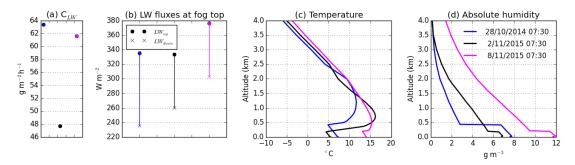
**Figure 6.** Comparison of three fog events at 07:30 UTC: (a)  $C_{LW}$  (defined in Sect. 2.1); (b) LW fluxes at fog top (cross is downwelling, circle is upwelling, thus length of vertical line indicates the (negative) LW budget at fog top). (c) Temperature and (d) humidity profiles estimated with the method described in Sect. 3.3. The fog top is located at the bottom of the sharp temperature inversion.
