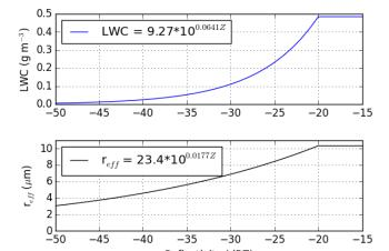
**Figure 2.** Empirical relationships between radar reflectivity (Z) and LWC and effective radius used in this study, based on Fox and Illingworth (1997).
