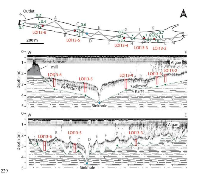
Figure 2. Navigation grid (grey lines), core locations (red dots), punctual sediment thickness measures (green dots) and acoustic images (200 kHz) of sedimentary infills within the Saint-Samson millstream. Grey letters refer to angles in the navigation grid. The dashed green line is an estimation of the karst-sediment interface depth based on measures of total sediment thickness.
