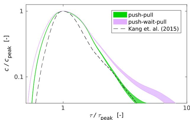
**Figure 3.** Inferred impulse-response breakthrough curves for the wethanalt experiments (experiments a and b in Table 1) obtained by deconvolution. The uncertainty associated with the unknown background salinity is represented by the thickening of the lines at late times. For comparison purposes, we also plot the breakthrough curve from the push-pull experiment by *Kang et al.* [2015] described in Table 1.
