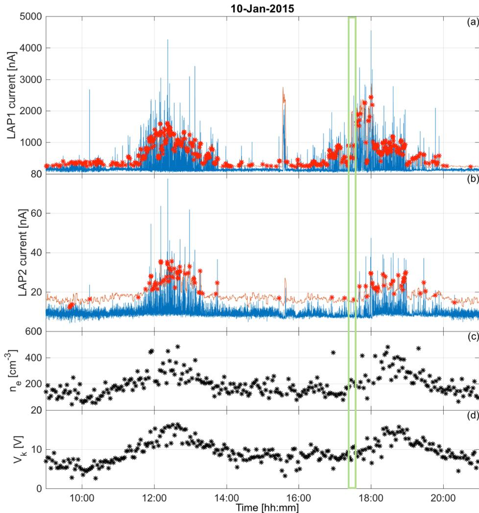
**Fig. 4.** Example of pulses in LAP1 (at +30 V, panel (a)) and LAP2 (at -30 V, panel (b)) current (blue). In red is shown the dynamic threshold used to define pulses, with red dots marking the pulses found by the algorithm. Panels (c) and (d) show sweep fit results for electron density and the negative of the spacecraft potential. The sign of the LAP2 current has been inverted, to show density increases as positive. The green box marks the interval zoomed into in Figure 5.
