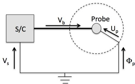
**Fig. 3.** Illustration of relevant potentials when there is no electric field in the unperturbed plasma. The bias voltage  $V_b$  is set by the instrument, while the other potentials result from the interaction of spacecraft, probe, and plasma. The ground potential can be seen as a point far away, or as what the potential would have been at the location of the spacecraft had it not been there.
