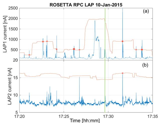
**Fig. 5.** Zoom in to part of the interval in Figure 4 to show details of pulses. The current here is sampled at 57.8 Hz, but very little structure is to be seen at timescales shorter than about a second. Blue is measured current and red is the dynamic threshold for pulse detection defined in the text. The vertical green line indicates the time of the sweep in Figure 6.
