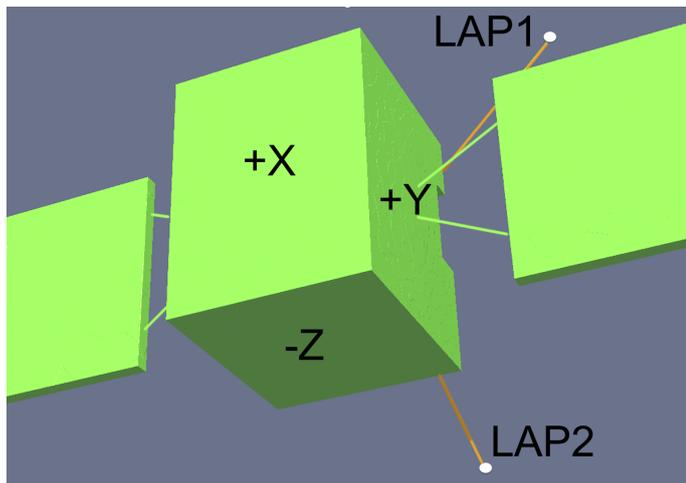
**Fig. 1.** Schematic showing the mounting of the LAP sensors. The LAP1 boom is in the YZ plane while the LAP2 boom is close to the XZ plane. Most of the time +Z pointed to the comet nucleus and +X was roughly in the solar direction. The solar panels and hence the Y axis were almost always perpendicular to the Sun. Not included is the high-gain antenna, mounted on the -Z side.
