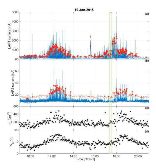
**Fig. 4.** Example of pulses in LAP1 (at +30 V, panel (a)) and LAP2 (at -30 V, panel (b)) current (blue). In red is shown the dynamic threshold used to define pulses, with red dots marking the pulses found by the algorithm. Panels (c) and (d) show sweep fit results for electron density and the negative of the spacecraft potential. The sign of the LAP2 current has been inverted, to show density increases as positive. The green box marks the interval zoomed into in Figure 5.
